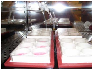
2D and 3D models are subjected to tension using the FlexCell device
